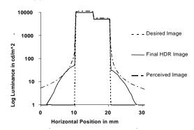
Figure 4. Comparison of display and eye introduced blur at a contrast boundaries of  $0 \text{cd/m}^2$  to  $10,000 \text{cd/m}^2$ ,  $10,000 \text{cd/m}^2$  to  $5,000 \text{cd/m}^2$  and  $5,000 \text{cd/m}^2$  to  $1 \text{cd/m}^2$ .
