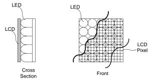
Figure 1. Layout of LED array behind color LCD
