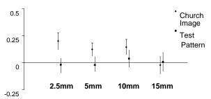
Figure 7. General quality ratings at increasing blur of the rear display.
